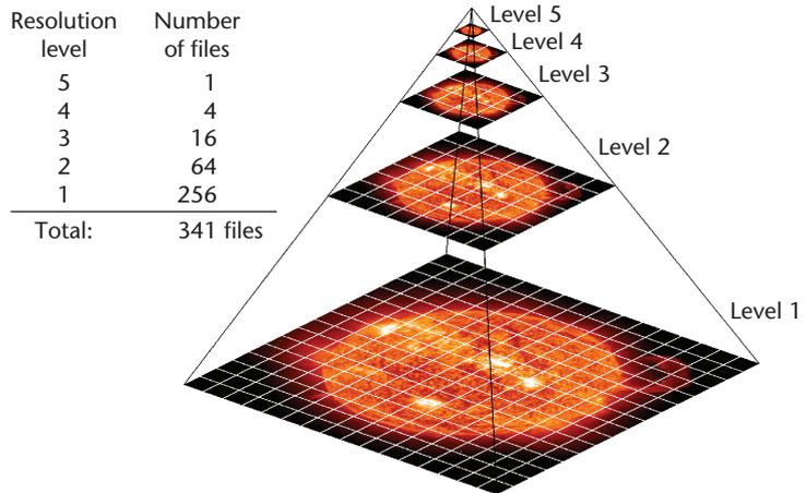
Figure 1. Image tile pyramid with five levels. In this example, a 16-megapixel image is tiled into 341 subimages that are  $256 \times 256$  pixels each.
