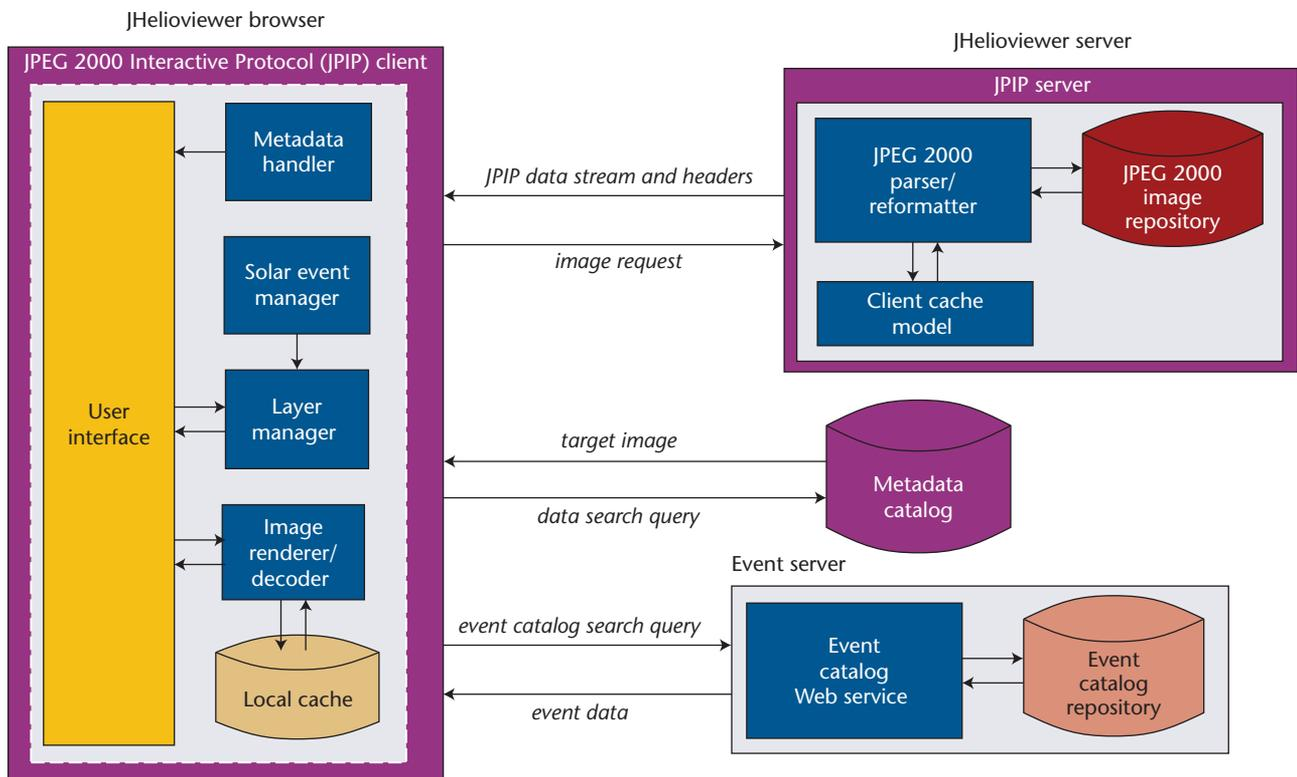
Figure 6. The JHelioviewer architecture. The architecture includes three basic parts—the browser (client), server, and solar-event server—that each include several key components.
