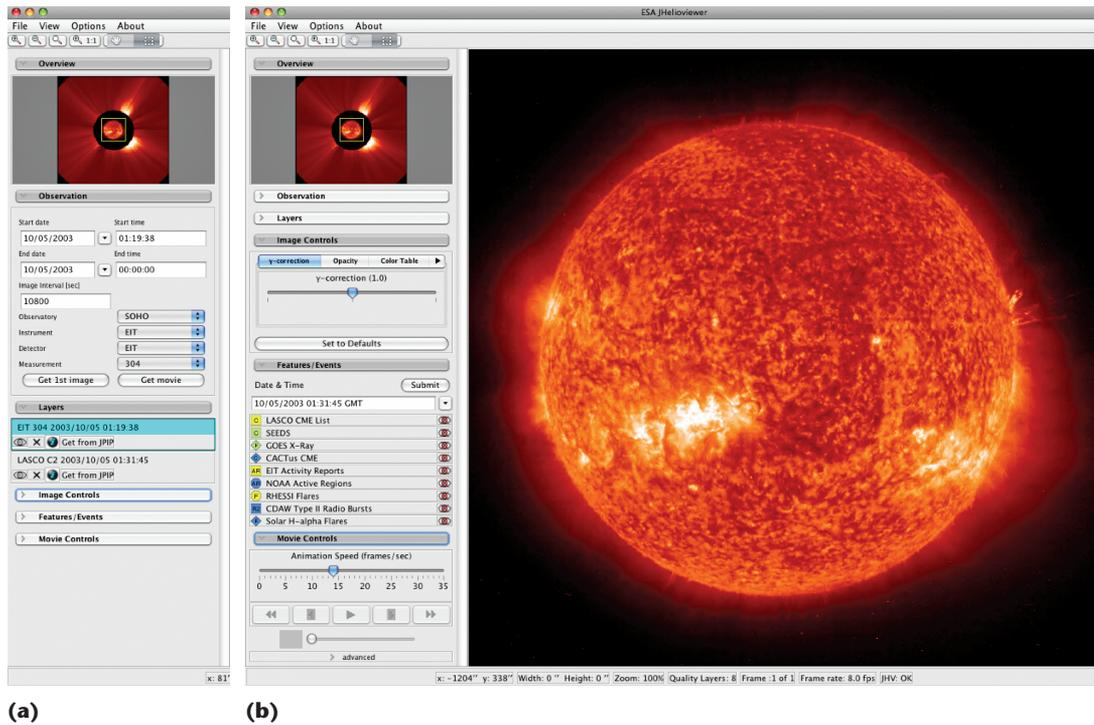
Figure 5. Screenshot of the JHelioviewer application. The left part of the application window has several expandable sections, which are shown in two panels for clarity. (a) The overview, database search interface, and layer manager. (b) The image controls, list of solar-event catalogs, and movie controls.
